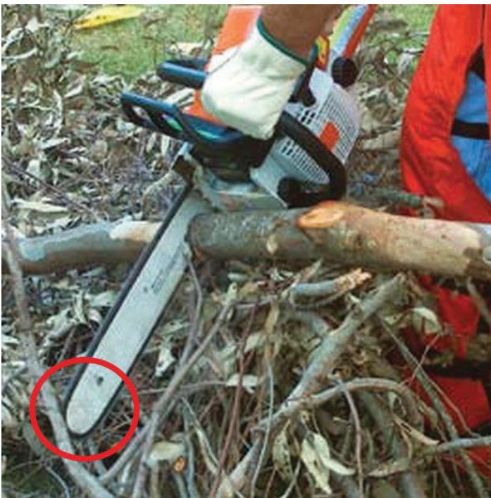
Figure 4. Do not cut with the upper tip of the saw—contact with other branches can cause kickback.
