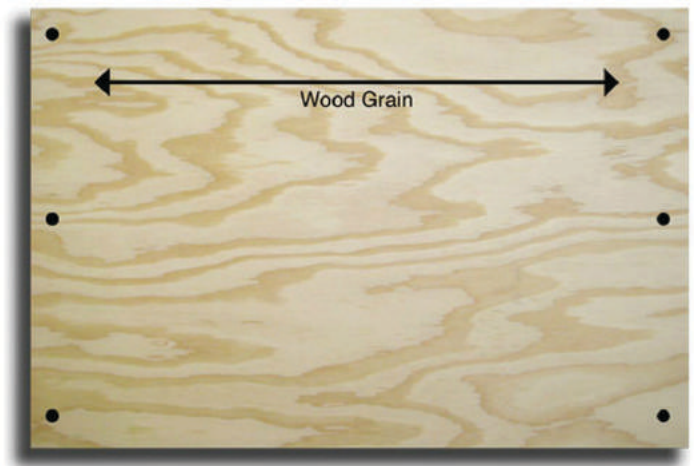
Figure 1. Plywood is strongest in the direction of its wood grain. Credits: Institute for Business & Home Safety
